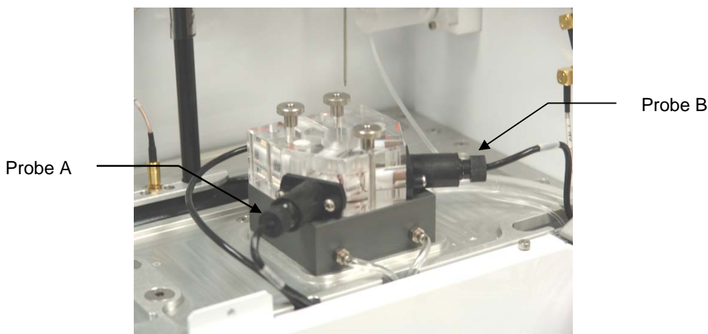
Probe A is always on the left when looking in from the side of the instrument Figure 4-4
